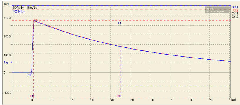
Figure 9: Lightning impulse behaviour – GIS type RGK 400DC [11]
